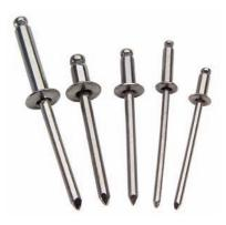
304 stainless steel open-end blind rivets are fabricated by stamping and are appropriate for outdoor and other applications where the rivet is subject to intermittent wetting. Zinc-plated steel open-end blind rivets are fabricated by cold-heading. Our open-end blind rivets conform to IFI Specification 114.
