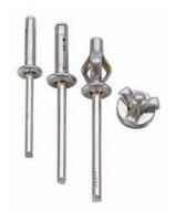
Aluminum trifold rivets are designed for the assembly of soft, brittle or thin materials. The trifold formation on the blind side applies the rivet's clamping force over an increased area, reducing the risk of cracking the parent material and compensating for irregular or oversized holes.
