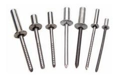
Closed-end blind rivets offer higher shear and tensile strengths, good vibration resistance, 100% mandrel ball retention and a water-resistant seal when installed in a defect-free hole.
